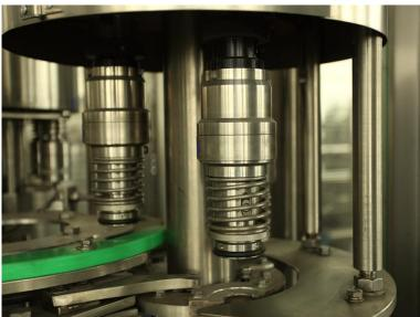
The stopper on the capping station jams the bottle neck, keeping the bottle upright and preventing rotation. The capping head keeps revolving and rotates on the capping machine, and realizes the actions of capping under the action of the cam, completing the entire capping process. The finished bottles are transferred from the capping machine to the bottle-out conveyor through the bottle-out dial wheel.
