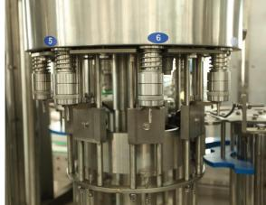
The rinsed bottle is blocked by the bottle neck tray and raised up by the cam, and then the filling valve is opened to start filling. After the filling valve is opened, the material completes the filling process through the filling valve. After the filling finishes, the bottle mouth drops and leaves the filling valve, and the bottle enters the capping machine through the bottle neck star wheel.
