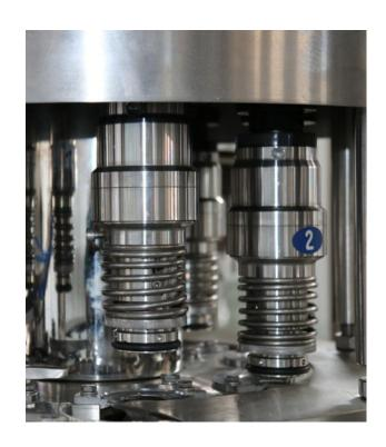
The stopper on the capping station jams the bottleneck, keeping the bottle upright and preventing rotation. The capping head keeps revolving and rotates on the capping machine, and realizes the actions of capping under the action of the cam, completing the entire capping process. The finished bottles are transferred from the capping machine to the bottle-out conveyor through the bottle-out dial wheel.
