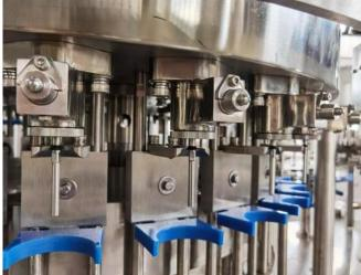
**High Precision Isobaric Filling Valve for Reference:**
