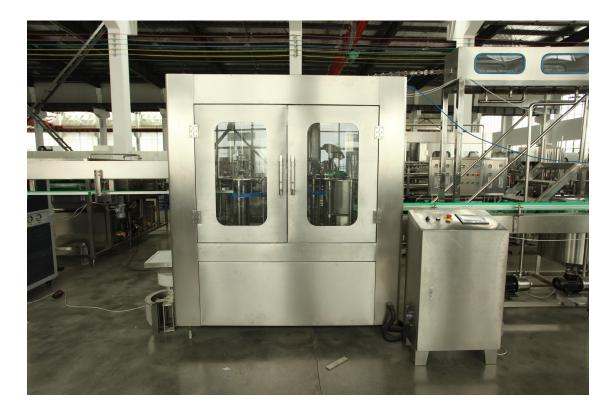
The fully automatic SGF series two-in-one juice filling machine is with stable structure, simple operation and high degree of automation. It is specially used for the production of PET bottled drinks of various specifications and bottle shapes. The parts in contact with the filling liquid are made of food-grade high quality stainless steel, which is hygienic.
